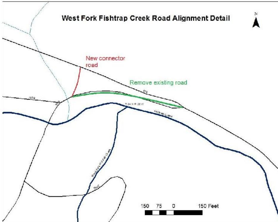
Map 1. Detail of the relocation of the junction of the West Fork Fishtrap road (#7609) with the main Fishtrap road (#516). The project will maintain motorized access while improving stream conditions at the confluence of Fishtrap Creek and West Fork Fishtrap Creek.
