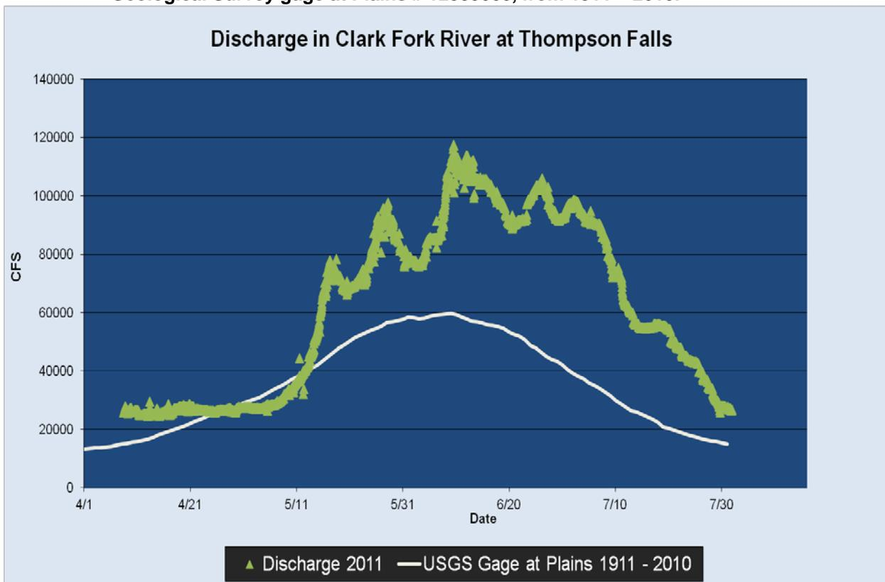
**Figure 6-3: Mean daily discharge in the Clark Fork River from April 1 to July 31 in each of the years when TDG data has been collected at the Thompson Falls Hydroelectric Project site. Data collected at the U.S. Geological Survey gage station at Plains, Montana, Station # 12389000.**
