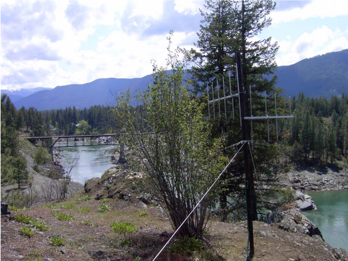
Photo 5. Antenna 1 of Hilltop telemetry station. Antenna 1 faces upstream on the mainstem Clark Fork River toward the viewable bridge. Note that the antenna facing towards the right was not used.
