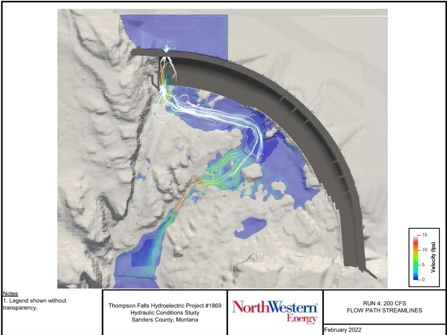
Figure 3-24. Run 4: 200 cfs Plan and Profile
