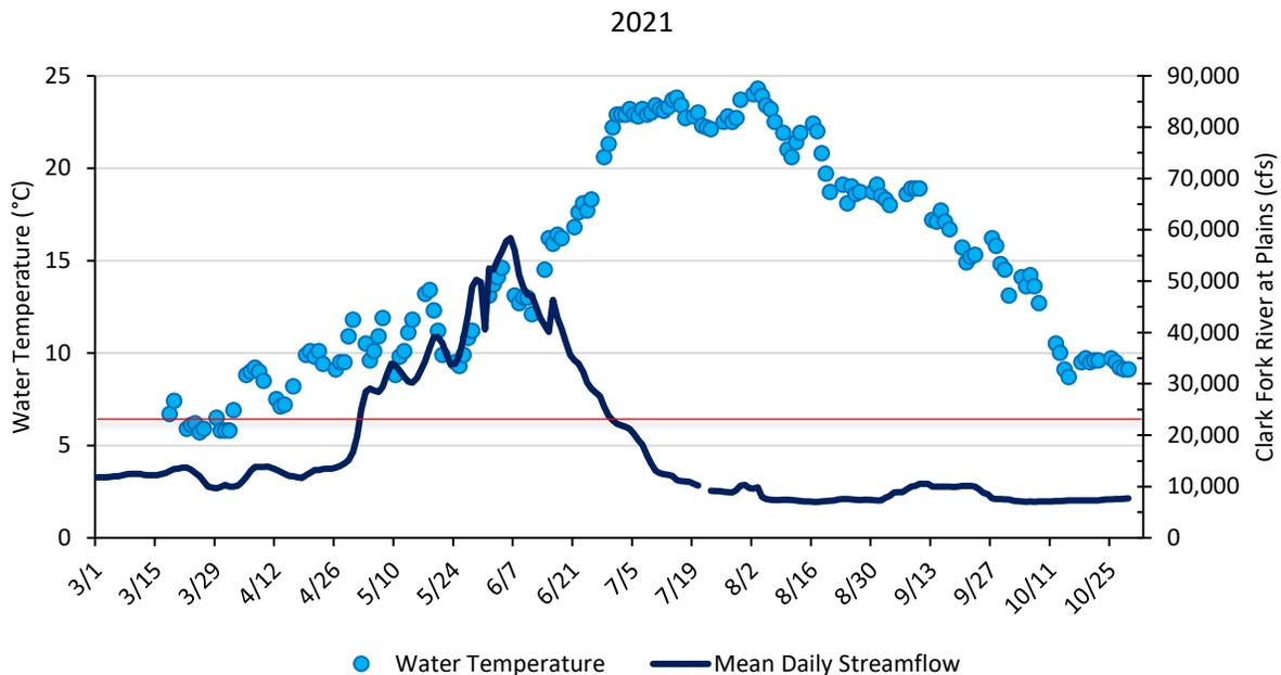
**Figure 3-2. Mean Daily Streamflow in the Clark Fork River near Plains (USGS #12389000), and Water Temperature Recorded at the Thompson Falls Upstream Fish Passage Facility, March 1 to October 26, 2022.**
