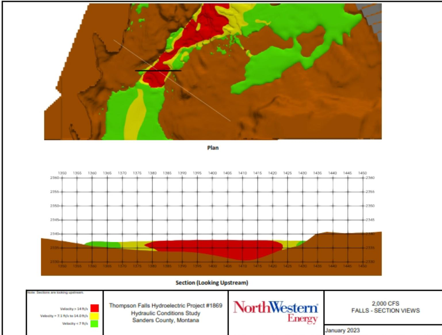
Figure 3-29. Model Scenario, 2,000 cfs. Cross-section at the Fish Passage Facility Entrance.
