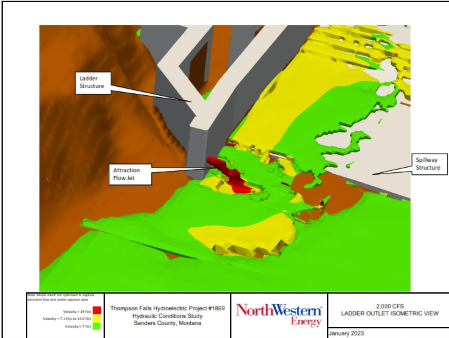
Figure 3-31 Flow Path Streamlines, 2,000 cfs at the Main Dam.
