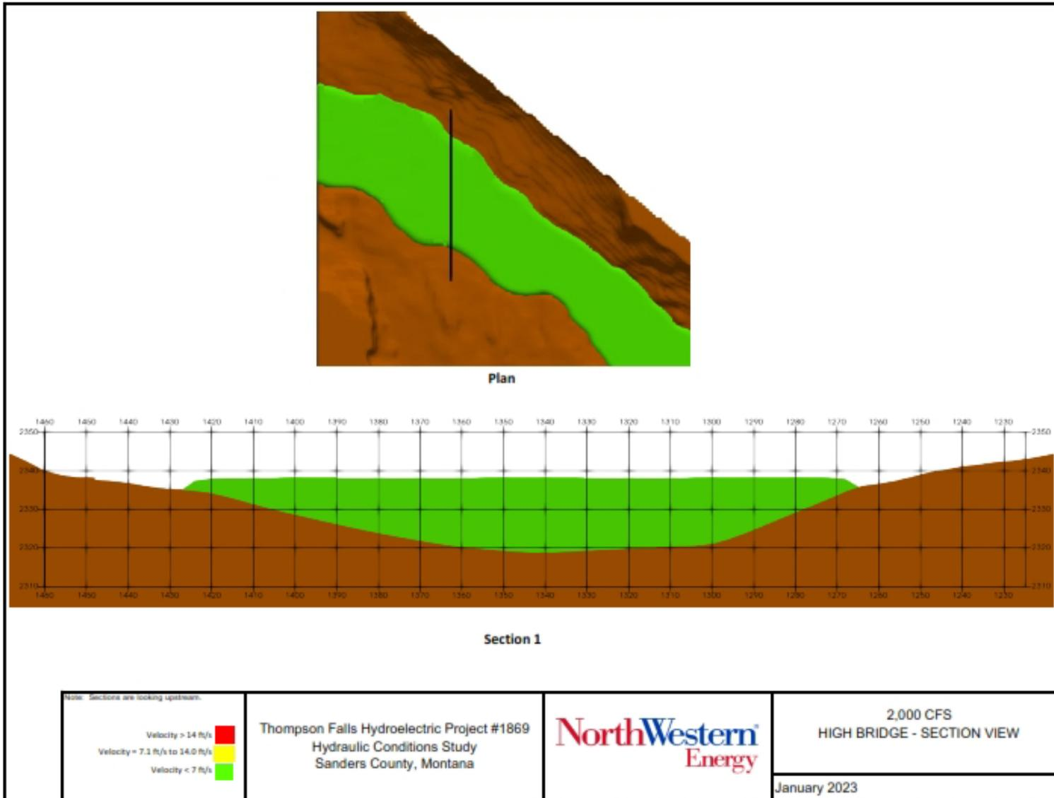
Figure 3-28. Model Scenario, 2,000 cfs. Cross-section at the Falls.
