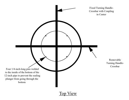
**Figure 27**-. Schematic of 12-inch diameter substrate sampler, modeled after the original 6-inch diameter sampler developed by McNeil and Ahnell (1964).
