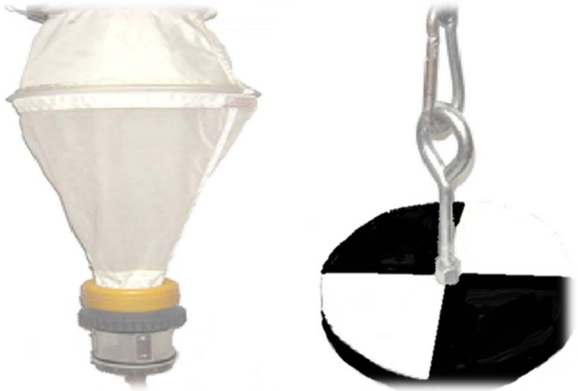
Figure 16. A Wisconsin plankton net (left) and Secchi disk (right) used to collect zooplankton and measure light penetration, respectively, in Hebgen Reservoir.
