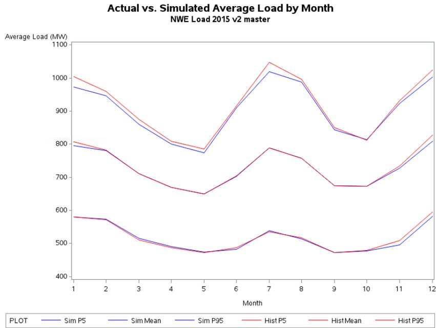
Figure 3. Backcast simulated (blue) load compared to 2015 NWE customer load (red). Simulated load closely follows the shape and distribution of load probabilities.
