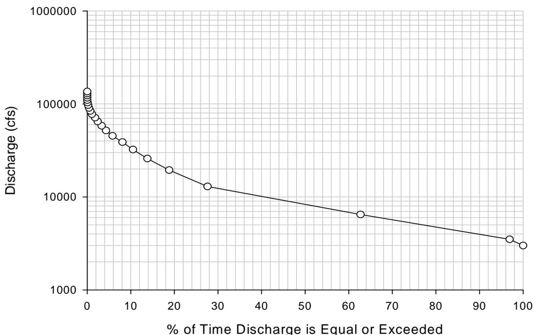
Figure 5 – River Discharge Exceedance Curve.
